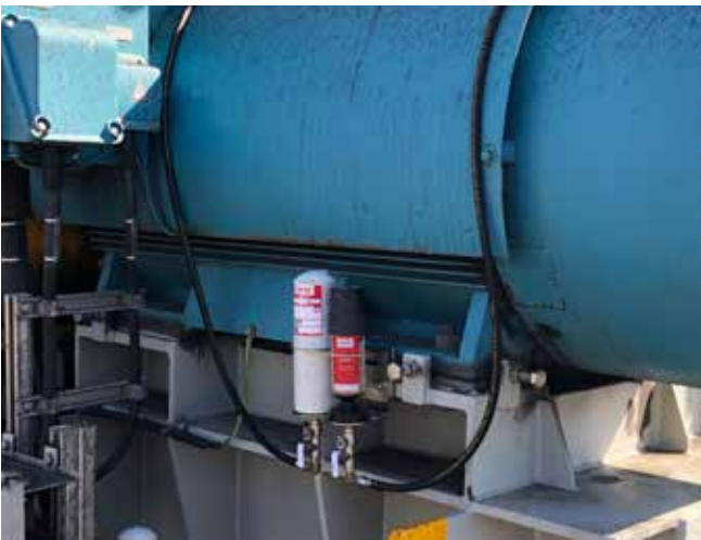
Application Electric motor Lubricator perma STAR VARIO 250cm 3 Installation kit K230C
