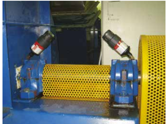
Application Fan support bearings Lubricator perma STAR VARIO 120cm 3 Installation kit Direct mount
