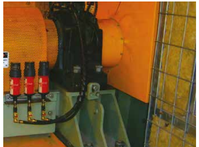
Application Fan support bearings Lubricator perma STAR VARIO 250cm 3 Installation kit K330
