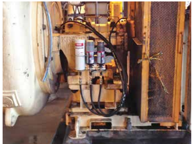
Application Labyrinth seals and gland seal Lubricator perma STAR VARIO 250cm 3 Installation kit K365C
