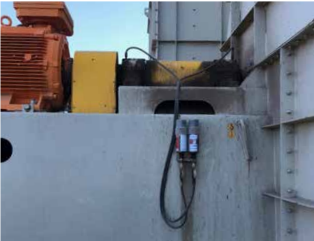
Application Fan support bearings Lubricator perma STAR VARIO 250cm 3 Installation kit K230
