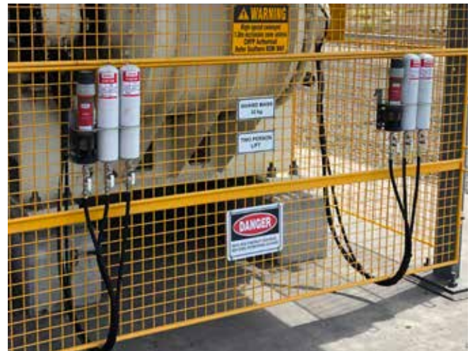
Application Conveyor pulley bearings and seals Lubricator perma STAR VARIO 500cm 3 Installation kit K3CHCX
