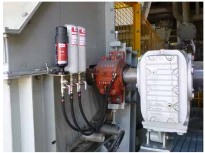
Application Conveyor pulley bearing and seal Lubricator perma STAR VARIO 250 cm 3 Installation kit K330
