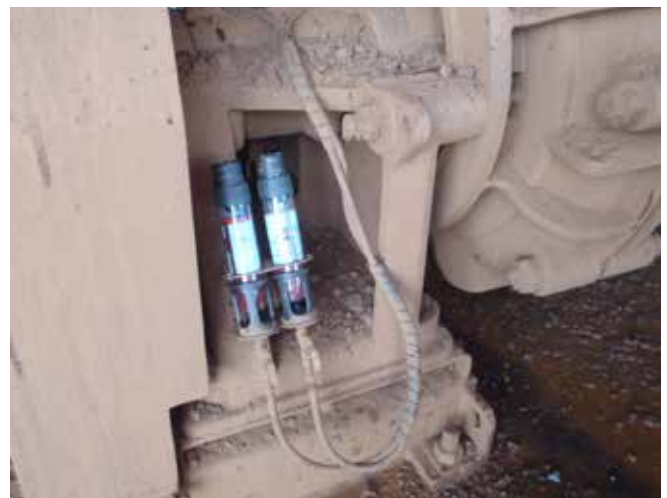
Application Labyrinth seals Lubricator perma STAR VARIO 500 cm 3 Installation kit K265CX
