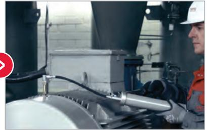
Pre-fill lubrication point, connecting parts and any grease lines with same lubricant as used in lubrication system
