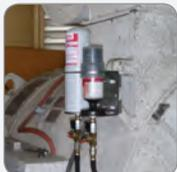
**Pressure build-up to 6 bar allows remote mounting up to 5 m**
