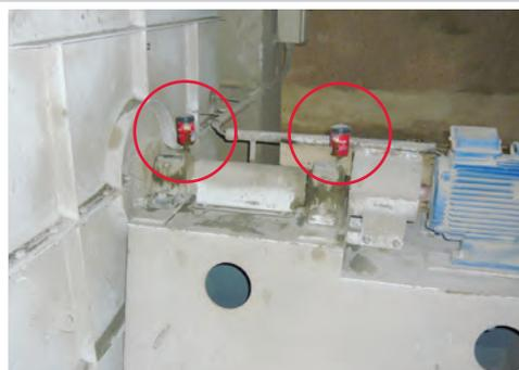
Lubrication of pillow block bearing on a fan drive shaft
