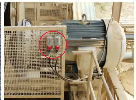
Remote lubrication of electric motor
