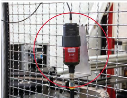
Automatic lubrication of a sliding guide
