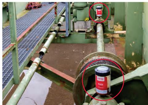
Roller bearing lubrication on a scraper
