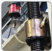
**Pressure build-up to 6 bar allows remote mounting up to 5 m**
