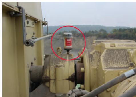
Roller bearing lubrication on the hot vertical bucket conveyor
