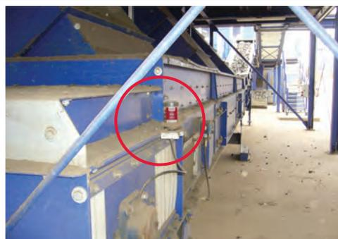
Flange bearing lubrication on a conveyor
