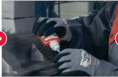
Apply thread sealant (e.g. Loctite® 243™) to all connecting parts, screw in reducer
