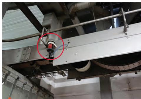
Chain lubrication on transport system box ejector
