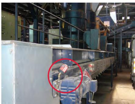
Flange bearing lubrication on a conveyor
