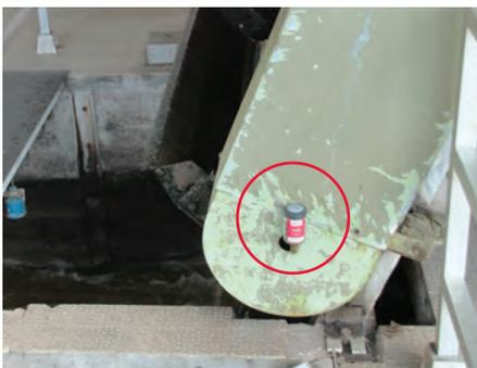
Roller bearing lubrication on a chain guide roller
