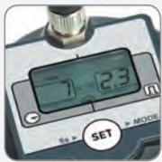
**LCD display with push button shows discharge settings, LC size and operating status**
