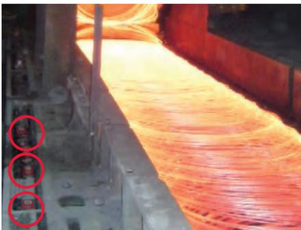
Drive chain lubrication (bolt stock conveyor)
