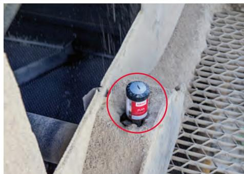
Lubrication of pillow block bearing on grit and sand screen
