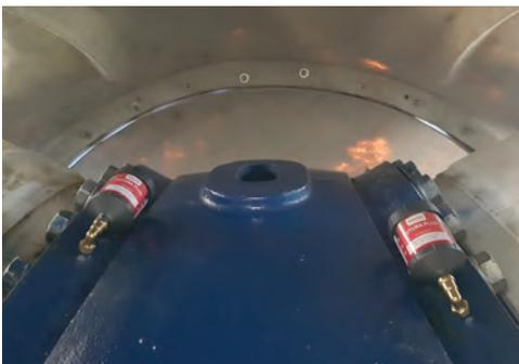
Blade bearing lubrication
