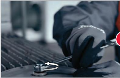
Clean the lubrication point, remove grease fitting
